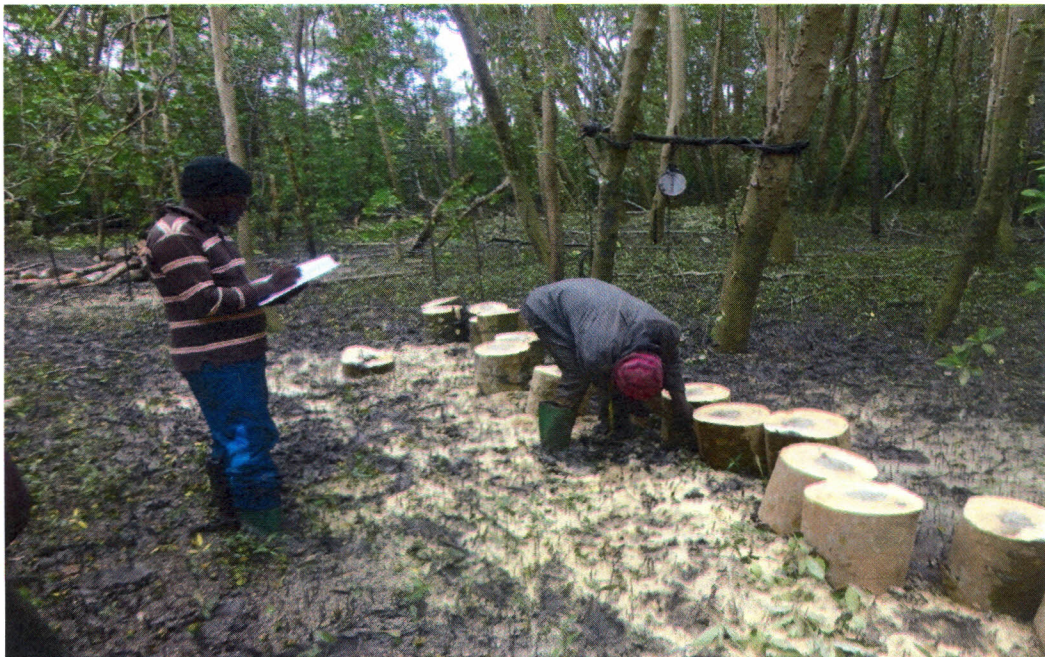
Plate 2: Recording diameters of billets before weighing in Rufiji River Delta, Tanzania (Photo: Lupembe, 2013)
